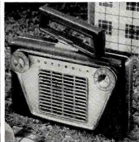
THIS new Motorola portable includes swivel handle that serves as antenna.
